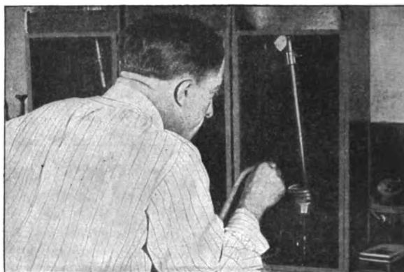
The Flash Test, Which Is One Important Indicative of an Oil's Suitability
